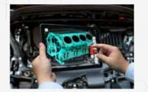
SuPAR is an augmented reality software that works as an Innovative Visual Quality Inspection Tool for remote inspection, rapid error detection and digital communication. Basically, you match the actual part with the details of the CAD drawing in real time whereby you can immediately report the findings. This interactive mobile inspection tool is most suitable for quality checks and geometry inspections in the automotive industry.
