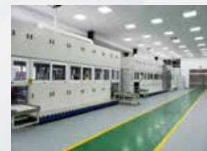
Fluorescent Penetrant Inspection (FPI)
