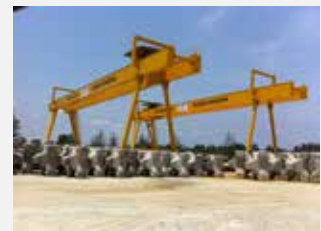
A-SHAPED GANTRY CRANE
